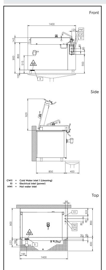
**Electric** Supply voltage: 400 V/3N ph/50/60 Hz Total Watts: 20.6 kW Installation: FS on concrete base;FS on feet;On base;Standing Type of installation:
